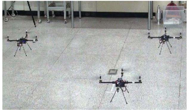
**Figure 16.** Three quadrotors in an experiment for an online task assignment algorithm.
