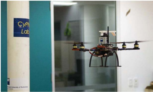
**Figure 15.** Mikrokopter-based quadrotor equipped with Gumstix and LRF [32].
