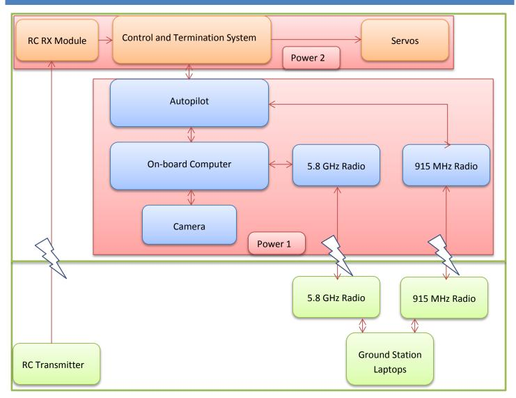
**Autopilot** – The autopilot will be based on the PX4 hardware platform, running the open source APM:Plane software. The primary connection to the Ground Control Station (GCS) will be via a low-bandwidth 915MHz telemetry and control radio link. A secondary connection to the 5.8 GHz high bandwidth link via the on-board computer will allow for redundancy.
