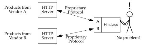
Protocol handlers get installed in a sequence similar to how content handlers get installed (see Dynamic types above): HOTJAVA is given a reference to an object (a URL). If the handler for that protocol is already loaded, it is used. If not, HOTJAVA searches, first the local system and then the system that is the target of the URL, for the protocol needed to interact with the object.
