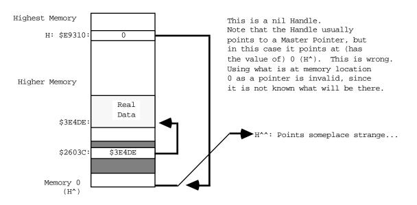
If the memory at 0 contains an odd number (numerically odd), then using it as a pointer will cause a system error with ID=2. This can be very useful, since that tells you exactly where the program is using this illegal handle, making it easy to fix. Unfortunately, there are cases where it is appropriate to pass a nil handle to ROM routines (such as GetScrap). These cases are rare, and it is **never** legal to read from or write to a nil handle.
