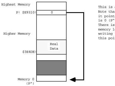
This is a nil Pointer. Note that the memory that it points to (the address) is 0 (P<sup>^</sup>). This is wrong. There is no valid data at memory location 0. Any writing to or reading from this pointer is a bug. nil handles are related to the problem, since a handle is merely the address of a pointer (or a pointer to a pointer). An example of what a normal handle might look like is:
