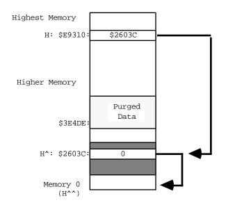
This is an Empty Handle. Note that the handle itself has a valid Master Pointer address in it \$2603C (H^). The Master Pointer is nil however, which is the address of location 0 in memory. It is wrong to use the Master Pointer in this case, although there are cases where using the Handle itself is valid.
