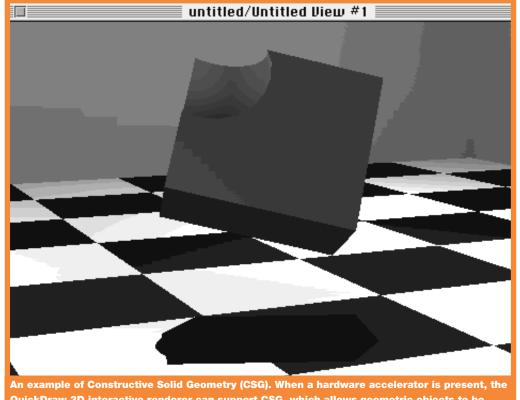
QuickDraw 3D interactive renderer can support CSG, which allows geometric objects to be "added" and "subtracted." The object pictured here is a cube that has part of a sphere subtracted from it.
