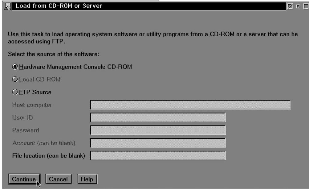
Figure 6. Selecting the source of the software
