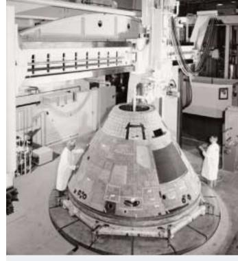
Run by an IBM System/360, a massive turret lathe shapes a heat shield for an Apollo spacecraft.
