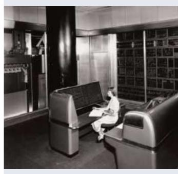
IBM's SSEC super calculator pointed up a critical problem: electro-mechanical input, output, and memory sources could not keep up with the new computing speeds.
