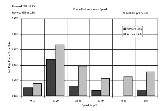
**Figure 5-1. Frame Error Rate Performance As a Function of Speed.** Power control, wideband modulation interleaving, and error control combine to limit error rates for all ranges of vehicle velocity.
