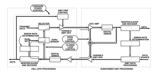
**Figure 3-2. Power Control in CDMA.** Fast open loop and closed loop control maintains the reverse link transmit power at a selectable level. A slower loop limits the forward link to only that power required.
