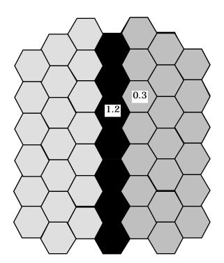
**Figure 4-2.** Unequal Cell Loading. When surrounding cells are lightly loaded, the capacity of heavily loaded cells can be increased. For the 30% surrounding capacity shown, the loaded cells are at 120% capacity.
