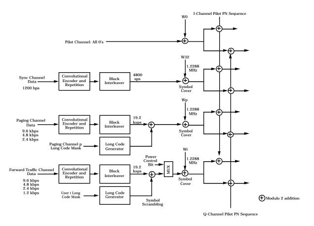
**Figure 4-4. Forward Link Channelization.** Forward link channels share a common pseudo-noise modulation, but are individually identified by the assigned Walsh functions (W0-W63). This allows flexible allocation of channels to paging for traffic channels.
