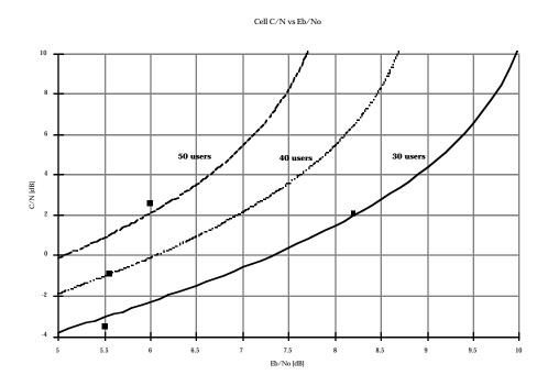
Figure 5-3. Limits in Sector Capacity Induced for Higher Required  $E_b/N_0$ . There has been close agreement between measurements and predicted Carrier--to -Noise ratios for a variety of capacity levels.
