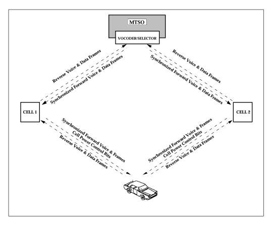
**Figure 3-3.** Active Links During Handoff. Following notification by the subscriber which identifies the desired new cell, the MTSO activates the new cell and communication is supported through both cells until the subscriber notifies the MTSO that one of the links is no longer useful.
