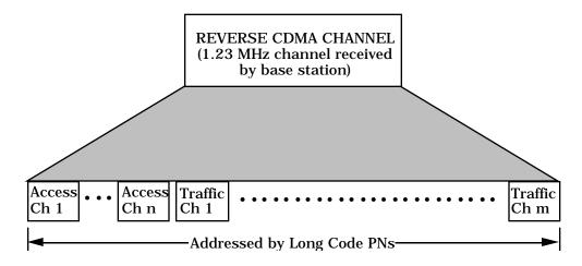
**Figure 4-6.** Reverse CDMA Channels Received at a Base Station. Reverse link channels comprise zero to 32 access channels and up to 64 traffic channels per paging channel. The channels can be distinguished by the subscriber unique PN code.
