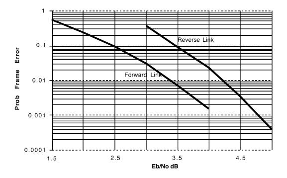
**Figure 4-1.** Performance of the Forward and Reverse Links on a Gaussian Channel. Tested  $E_b/N_0$  performance of both links shows the power of the modulation, interleaving, and error processing techniques employed. With power control, this results in a lower subscriber transmit power requirement.
