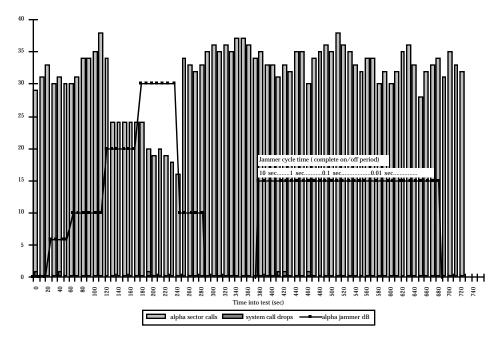
**Figure 5-4.** The Results of Injected Interference During the Field Tests. Total system tests showed the effectiveness of power control and handoff in reaction to unanticipated interference. Calls are shifted from cell to cell without losing calls as local conditions change.
