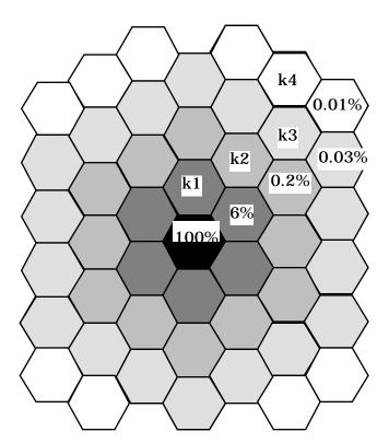
**Figure 3-4.** Interference Contributions From Neighboring Cells. Significant contribution to interference seen by a cell as a result of activity in other cells is limited to the first tier of cells surrounding the cell.
