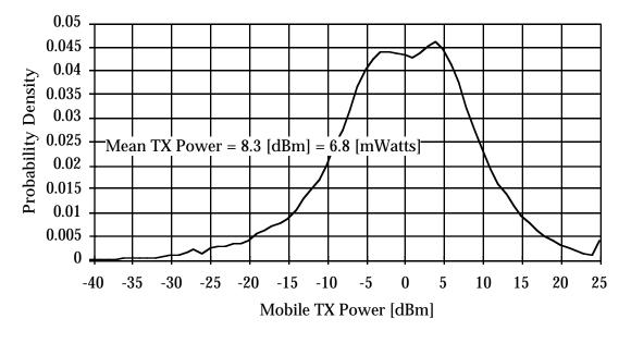
Mobile TX Power Statistics of Capacity Tests
