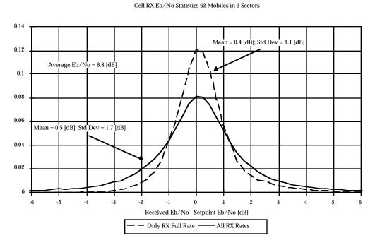
**Figure 5-2. Results of Power Control During Field Tests.** Field trials show a 1.7 dB standard deviation for power control of cell site received power in the variable data rate case. The full rate case is even better (1.1 dB).
