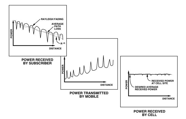
**Figure 4-7.** Effects of Power Control for the Reverse Link. The power control modifies the subscriber transmit power to provide nearly constant received power at the cell. The subscriber sees both variable average path loss and possible Rayleigh fading.
