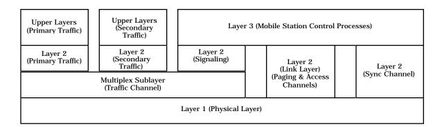
**Figure 4-8.** Mobile Station and Base Station Layering. The basic CDMA protocol is supported by the functions shown in Layers 1 through 3 (plus the multiplex layer). Individual services access the system through Level 2 to the multiplex Layer.
