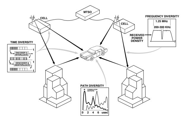
**Figure 3-1.** Diversity Processes in CDMA. The reception from two different cells, wide band, signal structure, along with the capabilities of the rake receiver allow CDMA three forms of diversity in addition to the time diversity available in other digital systems.
