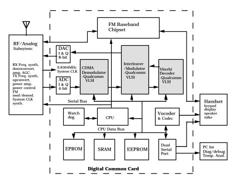
**Figure 4-11 Mobile Subsystem.** The subscriber unit comprises an analog section similar to current analog units and a digital processing section. The CDMA functions are contained in three (soon to become one) ASICs and the controller processor.
