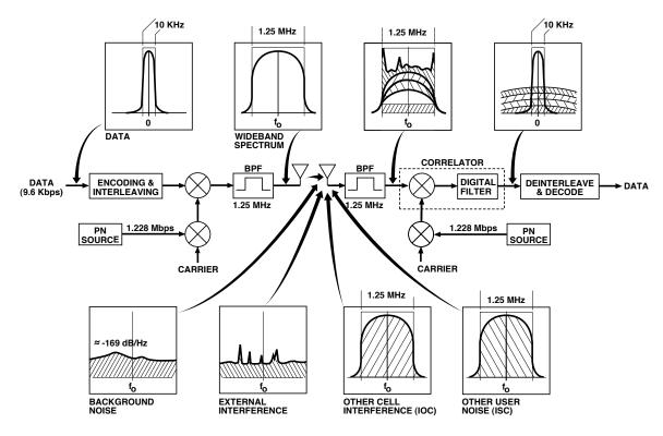
**Figure 2-2.** A View of the CDMA Concept. The desired signal is selected from four different sources of interference. The dominant source is system self-interference produced by other users of the same cell. This source is controlled by closed loop power control.
