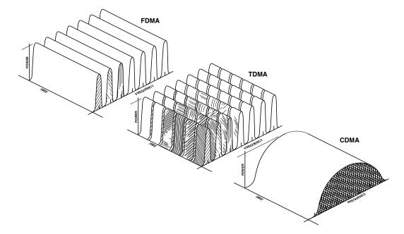
**Figure 2-1. Frequency and Time Domain Representations of FDMA, TDMA, and CDMA**. Unlike FDMA or TDMA, CDMA has multiple users simultaneously sharing the same wide band channel. Individual users are selected by correlation processing of the pseudonoise waveform.
