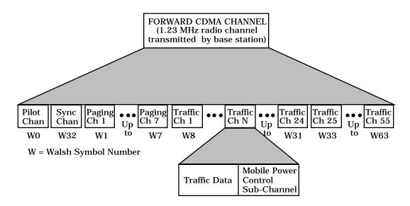
**Figure 4-5.** Forward CDMA Channels Transmitted by a Base Station. In addition to the pilot and sync channels, the forward link in each sector supports 62 channels that may be used for paging and traffic. Zero to seven channels are assigned to paging, the remainder are traffic channels.
