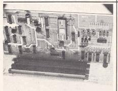
**1.** Central Processing Unit (CPU) Board. This double-sided board is the heart of the Altair 8800. It was designed around a powerful, byte oriented, variable word length processor—a complete central processing unit on a single LSI chip using n-channel, silicon gate MOS technology. The CPU board also contains the Altair System Clock—a standard TTL oscillator with a 2.000 MHz crystal as the feedback element.
