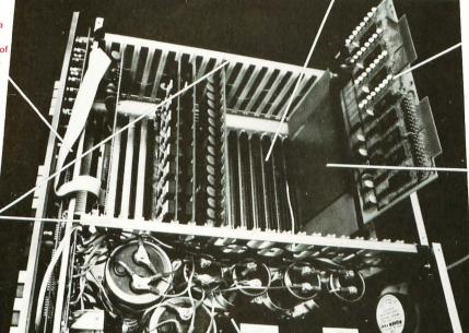
Special PIO Board configured with LEDs to monitor each bit of each of the 4 ports.
