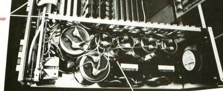
Heavy duty power supply (optional dual power supply shown.)
