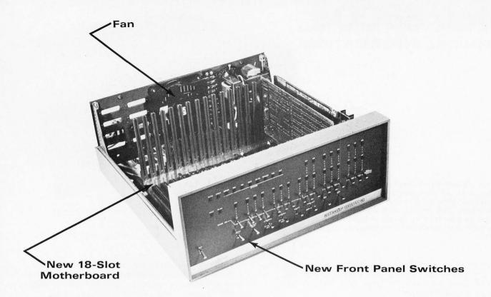
The four boards, along with the power supply, mount in an 18" deep x 17" wide x 7" high (45.7 x 43.2 x 17.7-cm) metal cabinet.
