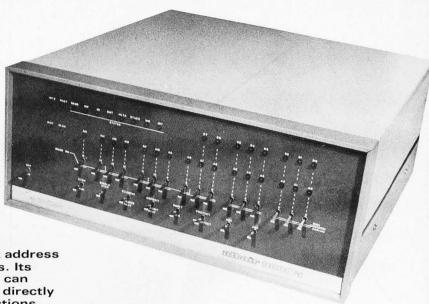
The Altair 8800a is a parallel 8-bit word/16-bit address computer with an instruction cycle time of 2  $\mu$ s. Its central processing unit is the 8080 LSI chip. It can accommodate 256 inputs and 256 outputs, all directly addressable, and has 78 basic machine instructions. It is capable of directly addressing up to 65,000 bytes of memory.
