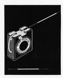
A new wire dispenser from OK Machine and Tool Company, 3455 Conner St, Bronx NY 10475, combines cutting and stripping ability in one unit. Wire is drawn out of the dispenser to the desired length, cut with the built-in plunger, and pulled through the stripping blades. Dispenser includes 50 feet (15 meters) of AWG 30 insulated solid copper wire available in four colors. People who use conventional wire wrap will find this to be an excellent addition to the tool kit.
