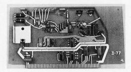
Pinnacle Products has announced a self-refreshing 4 channel digital to analog converter that is Altair bus compatible. Instructions are included for alternate connection to Digital Group Systems. Features include complete output port address decoding and a 3 state bus connection. The converter has eight bits of resolution and can be set to cover any range within -10 to 10 V. It oper-
