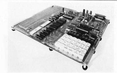
The 2 K bytes of 2142-type programmable memory can be doubled by implementing additional devices in the positions provided. There is room for 8 K bytes of program instructions using either or both of the keyboard and terminal software monitors included in the kit. There is a fully buffered system bus. Programs and data may be entered three ways: from the built-in keyboard; through a built-in serial communications interface; or via cable (SDK-C86) from
