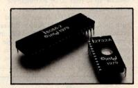
the 8089 input/output processor can be used in 8086-2 systems, acting as a coprocessor in the system, executing input/output programs concurrently with the 8086 execution of the main program. The 8086-2 is currently priced at \$200 in quantities of 100 and the 2732A EPROM is currently priced at \$570.
