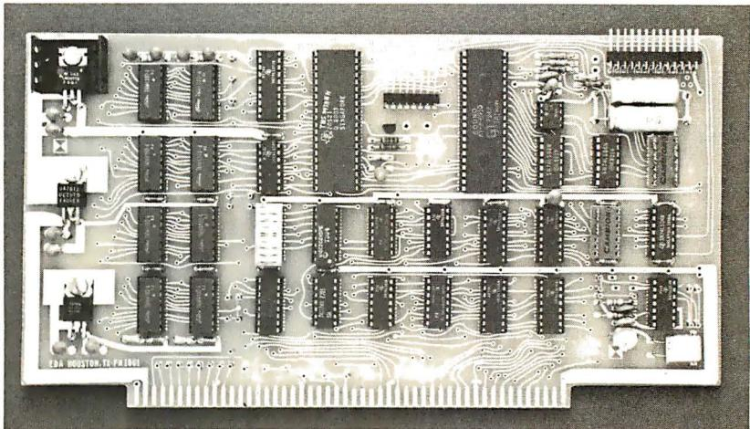
generator uses the Texas Instruments TMS9918A Video Display Processor and the General Instrument AY-3-8910 Programmable Sound Generator, and is compatible with Z80, 8085, and 8080 microprocessors on S-100 bus systems. Documentation in-
