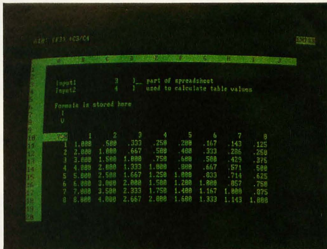
Photo 3: Two-dimensional table creation in 1-2-3. When it's given a spreadsheet, two lists of input values, input cells for both lists, and an output cell, 1-2-3 can automatically create a table that gives the output value for each combination of the two input values. Photos 3a and 3b show the spreadsheet before and after the command is given. The output function shown here is the ratio of the two input values.
