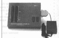
The ADC-1 serves as a real world interface for any computer or modem with a RS-232 serial port.
