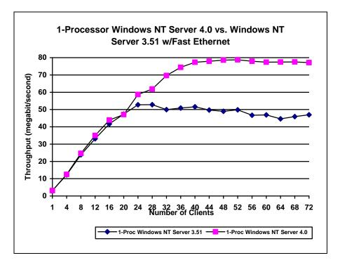
The hardware was a Compaq ProLiant 5000 server equipped with a single Pentium Pro 166 processor, 128MB RAM, a 4x2GB disk array, and a Fast Ethernet network interface card. Each test used up to 72 clients running Windows 95. The client machines were Pentium 100s with 16 MB of RAM. Windows NT Server 4.0 achieved a throughput of 77.12 megabits/second at 72 clients, an increase in file and print performance of more than 60 percent over Windows NT Server 3.51.
